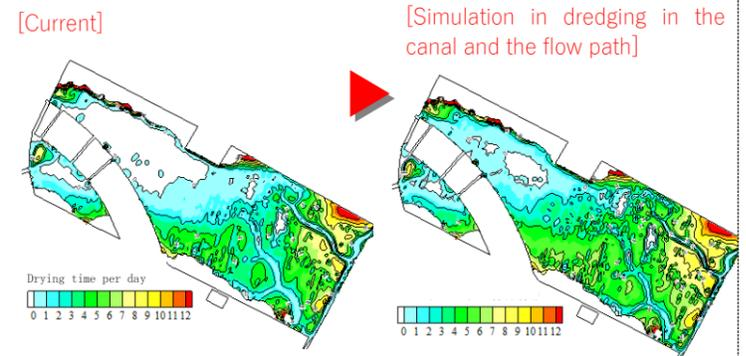
Calculated pattern of area and duration of exposure by numerical simulation
