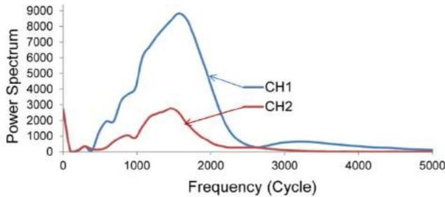
Fig.19 - Power spectrum of hammering:  $\phi$  6mm
