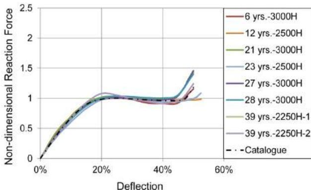
Fig. 4 - Performance of used fenders:  $H > 2000$ mm
