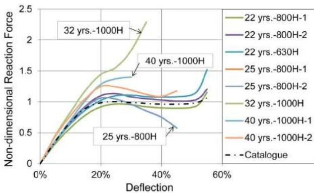
Fig. 2 - Performance of used fenders:  $H \leq 1000$ mm fender
