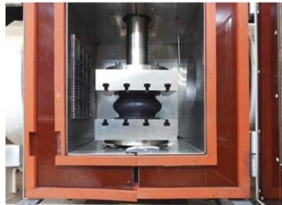
Fig.8 - Compression tester for miniature model
