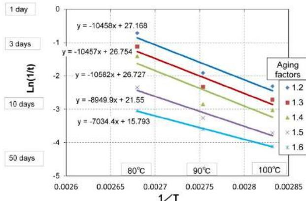
Fig.7 - Arrhenius plot of rubber sheet (Stress at 100% strain)
