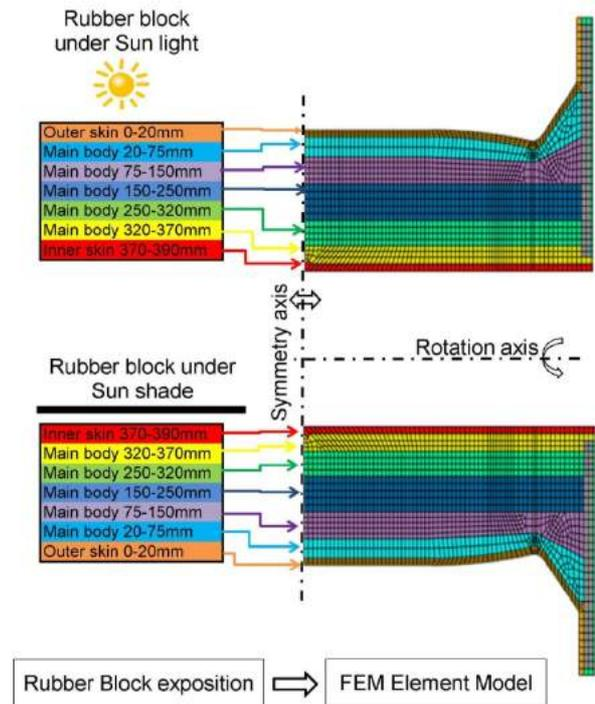
Fig. 13 - Exposition test of rubber for FEM elements
