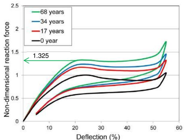
Fig.9 - Performance of miniature fender: 100H (Average of 2-3 compression cycles)
