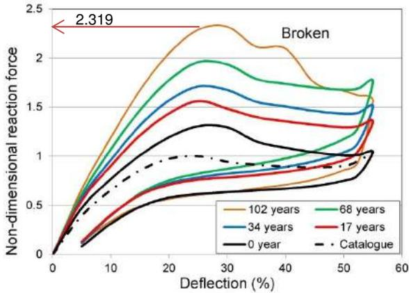
Fig. 10 - Performance of miniature fender: 100H (1st compression cycle)
