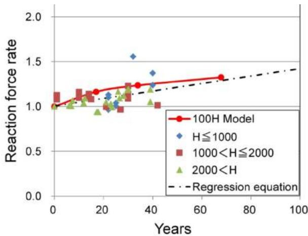
Fig. 11 - Reaction force rate: 100H Model (Average of 2-3 compression cycles)
