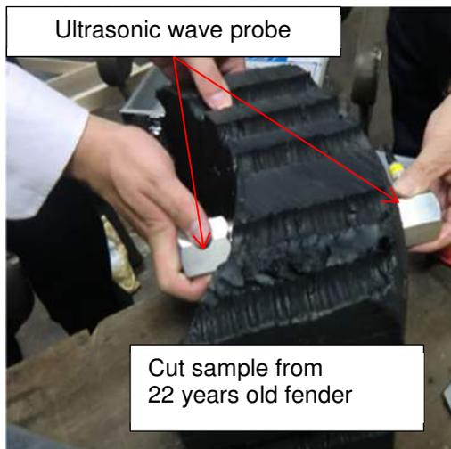
Fig.20 - Ultrasonic wave transmission through rubber
