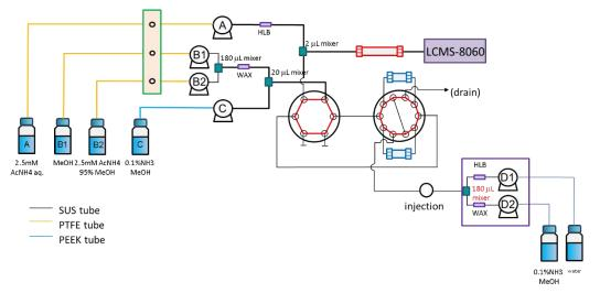
Fig. 1 Flow diagram of online-SPE-LC-MS/MS with multi-gradient eluent
