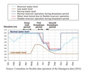
**Fig. 4.** Schematic diagram of flexible dam operation at Managawa dam.
