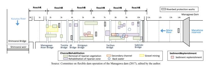
Fig. 7. Schematic diagram on managed flows, sediment replenishment, and channel rehabilitation in Managawa River.
