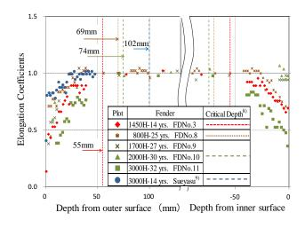
Fig.9 Elongation coefficients of returned fenders near surface (Upper side).
