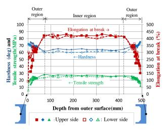
**Fig.6** Distribution of material properties of FD No.11: 3000H(R0-10) after 32 years.
