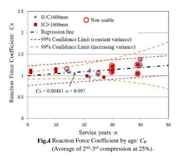
fenders, but it should be warned that there are nonvisible aging effects other than reaction force and 30 years is a reasonable time for replacing fenders.
