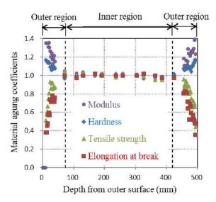
Fig.8 Distribution of material aging coefficient: FD No.11 3000H(R0-10), 32 years, Upper side.
