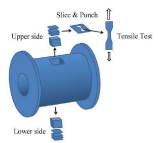
Fig. 5 Rubber sampling from returned fenders.
