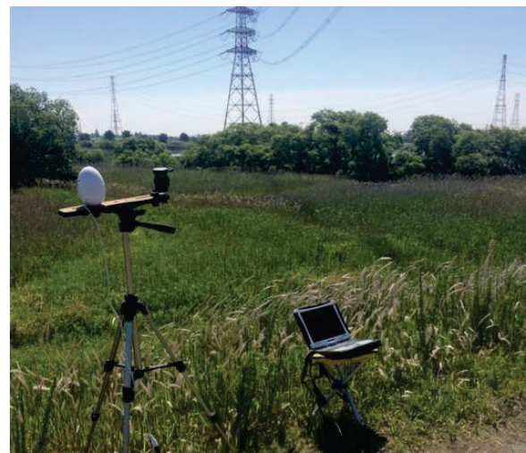
Fig. 3. Photo illustrating one of the three microphone arrays connected to a laptop computer at the recording site.
