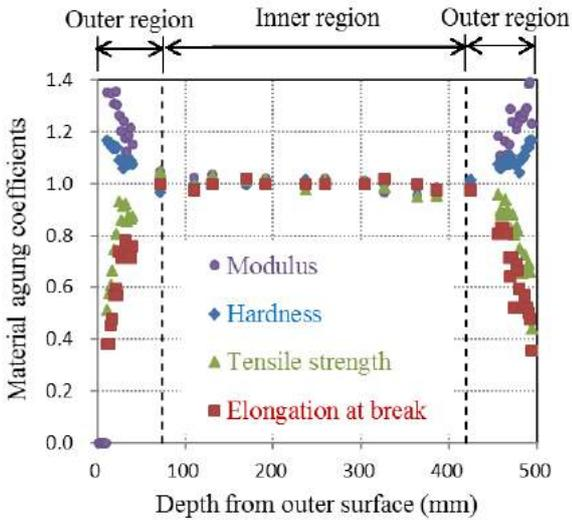
**Fig.8** Distribution of material aging coefficient: FD No.11 3000H(R0-10), 32 years, Upper side.
