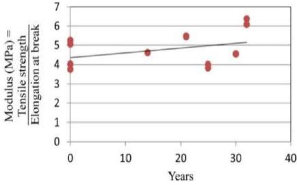
**Fig.7** Aging of modulus of inner region: (Average tensile strength) / (Average elongation at break).
