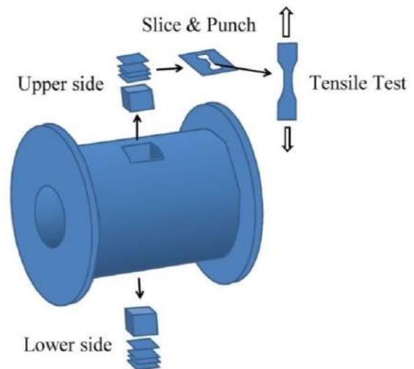
**Fig. 5** Rubber sampling from returned fenders.
