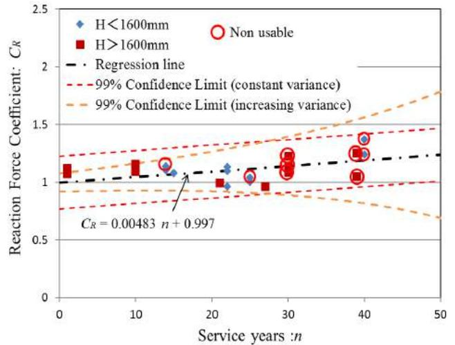
**Fig.4** Reaction Force Coefficient by age:  $C_R$
