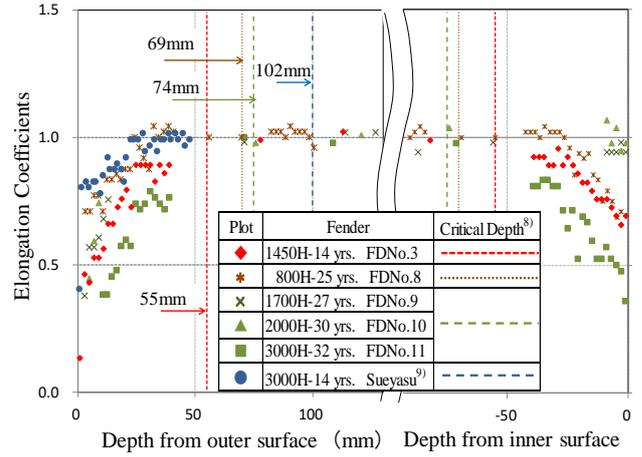
**Fig.9** Elongation coefficients of returned fenders near surface (Upper side).
