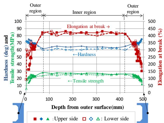
**Fig.6** Distribution of material properties of FD No.11: 3000H(R0-10) after 32 years.
