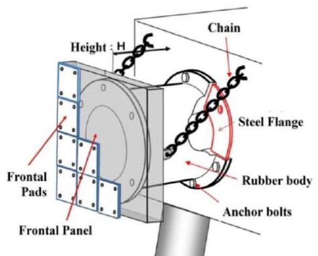
**Fig.1** The Circular Shaped Buckling (CSB) fender system.
