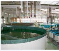
Equipped with outlets for seawater, groundwater and aeration supply to enable various experiments with aquatic organisms.
